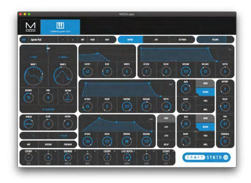
This is the main tab for patch design / editing. You will find oscillator, filter, envelope, LFO, arpeggiator, sustain, modulation and effects sections here.
