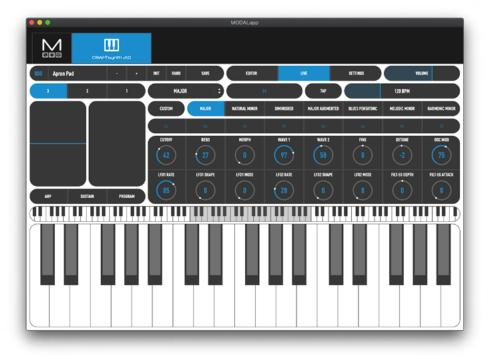
This page provides a MIDI controller for playing your CRAFTsynth 2.0 with access to keys, pitchbend and modwheel, arp and sustain settings and 16 assignable macro controls.
