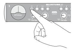
5. Speak into the microphone while watching the VU meter on the front panel and slowly turning the BlueTube DP V2 Input 1 Gain knob clockwise.
