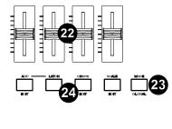
The Mode Button LED indicates which Mode the Function Buttons are in.
