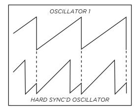
The sound can become aggressive, metallic, or even exhibit elements of comb filtering. Adding modulation to the frequency of a sync'd Oscillator can greatly enhance this effect. Moog One sets Oscillator 1 as the Master Oscillator by default. Use the **HARD SYNC** button to force the selected Oscillator(s) to sync to Oscillator 1.
