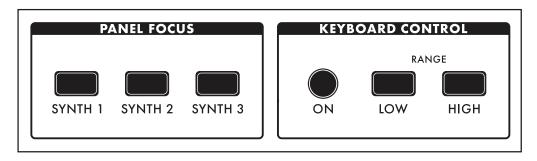
The active Synth is selected using the **SYNTH 1**, **2** and **3** buttons in the Panel Focus module, which allows the Front Panel knobs and buttons to only affect the currently selected Synth(s). Pressing any **SYNTH** button by itself will select just that one Synth. Holding one **SYNTH** button while pressing additional **SYNTH** buttons will select multiple Synths, and allow any tweaks or edits to be applied to all of the selected Synths simultaneously.
