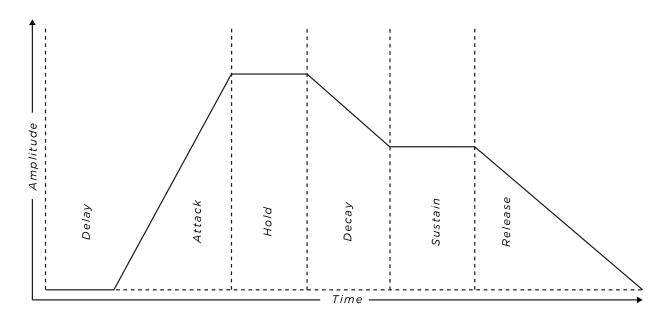
In this diagram, you can see how the Delay Time, Attack Time, Hold Time, Decay Time, Sustain Level, and Release Time work together to form a continuous control signal. The Envelope begins as the key is pressed, and the Release stage begins when the key is released. An external gate can also be used to trigger an Envelope.
