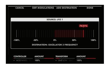
At this point, pressing the DONE Soft Button at the top of the screen will complete the modulation routing, or the CANCEL Soft Button can be used to exit this modulation screen without making the modulation route complete. The functions of the additional Soft Knobs and Soft Buttons are discussed elsewhere, in the MODULATION section.
