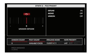
These onscreen parameters are accessed using the Master Encoder and the four Soft Knobs below the screen.
