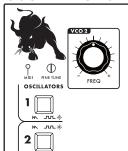
The Oscillators are the main sound source of the Minitaur. They create electronic vibrations that can be tuned and amplified into sound that we can hear. The Minitaur's VCOs can produce a total musical range of 6 octaves.
