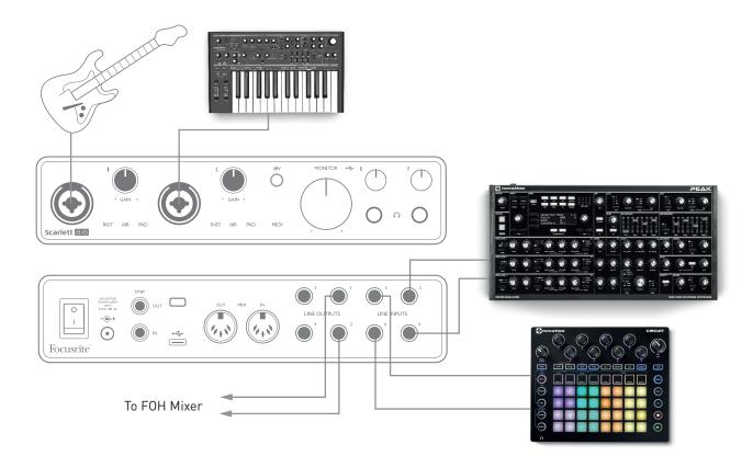
In the example illustrated, a guitar, stereo and mono synths and a electronic groovebox instrument are connected to the six analogue inputs of the Scarlett 8i6; Outputs 1 and 2 go to the main PA system. The player can set up a rough mix in Focusrite Control and then adjust the levels of the two mono sources against the stereo ones from the front panel.
