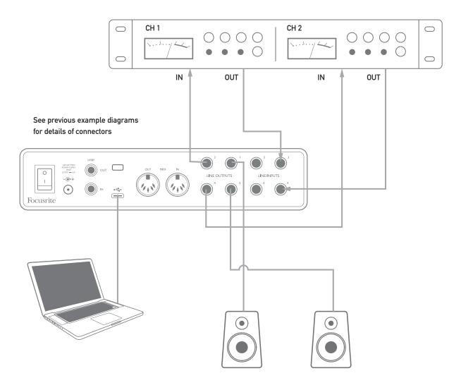
You can adjust the levels to and from the external processor from Focusrite Control, if necessary.
