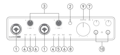
The front panel includes input connectors for Mic, Line and Instrument signals, the input gain and monitoring controls, and headphones sockets.
