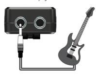
**4** Connect an amplifier to the amp output via an instrument cable with a ¼" TS connector.
