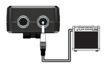
Move the THRU/FX switch to the FX position to hear the processed guitar or bass sound from the app in your mobile device.
