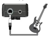
• Connect an amplifier to the amp output via an instrument cable with a ¼" TS connector.
