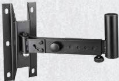
PA S11 Supporto orientabile e allungabile da muro Adjustable and extendable wall support Length: Min 320 - Max 420 H/V angle: 180° - max 60° Load capacity: max 50 Kg
