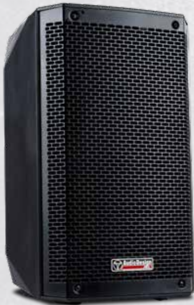
X-Jam 10 Diffusore attivo professionale a 2 vie 2 Way professional active enclosure Woofer: 10"/250 mm - Driver V/C 34 mm Max Power: 1.000 W SPL Max: 123 dB 1 m Peso Kg 9,8 - Dimensioni 30x31x51 cm
