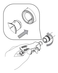
4 Attach the counterweight onto the tonearm.
