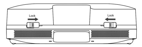
To remove the dust cover, slide the buckles to unlock them, and tip the front cover back to open it. Remove the tabs from the grooves to take off the cover.
