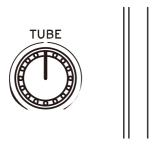
**TUBE knob:** Adjusts the depth of the vacuum tube (Nutube) effect. Turn this clockwise to increase the effect, and counterclockwise to decrease it.
