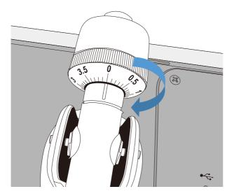
3 Turn the counterweight counterclockwise and set it to a needle pressure that's suitable for the cartridge.
