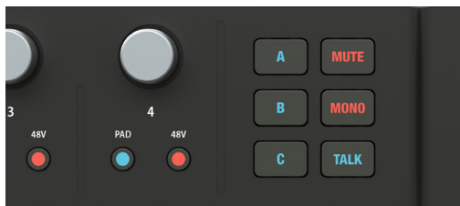
Figure 5-5: A/B/C Mode and Monitor controls on the front panel.
