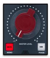
Using the LEVEL PRESET OPTIONS: The RAM SYSTEM 5000 has the ability to store 2 different level presets, which override the Red Level knob position. Pressing SHIFT + OUT 5 (Level Preset) will ask for which of the 2 presets it should be stored to (1 or 2). Confirmation is given by pressing the corresponding key, OUT 1 (Level Preset 1) or OUT 2 (Level Preset 2). Pressing SHIFT + OUT 1 (Level Preset 1) will make the monitoring level that of the stored preset, same for Preset 2.
