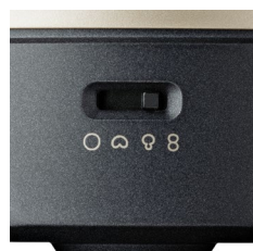
Figure 1: Selector for polar patterns
